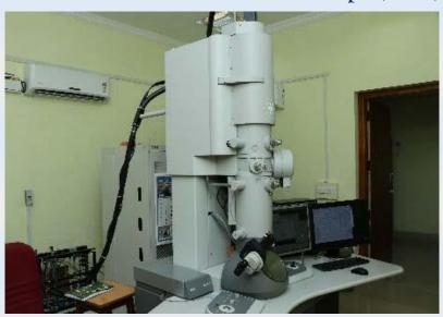
The FEI Tecnai G<sup>2</sup> 20 S-TWIN TEM is designed to offer an imaging and analysis solution for life sciences, materials sciences, nanotechnology, and the semiconductor and data storage industries. A wide range of functionality and techniques is available and can be combined on the Tecnai G2 20 S-TWIN TEM, to name a few: high contrast imaging, HR-TEM and SAED, using embedded detectors and components like BF/DF, CCD and corrected optics.
